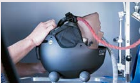
Test machines for vertical drops
